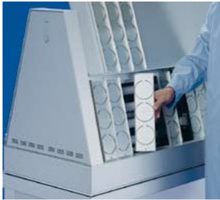
Test specimens are mounted in convenient snap-ring holders.
